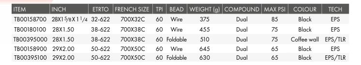
The CST Pika is a dirt road tire built to handle the ever-changing conditions encountered during your daily commute or a weekend gravel grind. The tire has ramped centre knobs for a smooth, fast ride, while the shoulder tread features U-shaped knobs designed to give you confidence in the turns. The CST Pika comes in 700x38c and is equipped with dual compound tread, Defender Cobweb protection and wire bead.
