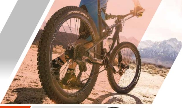
The Rock Hawk from CST features an aggressive tread pattern with large, wellspaced lugs. This spacing allows the tire to shed mud and other debris on mountain bike trails with varying conditions. In order to help reduce rolling resistance, the center knobs have been ramped. The Rock Hawk is available with a wire bead or folding bead with Defender Cobweb puncture
